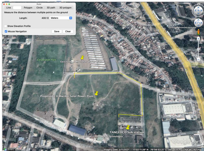
Figure 4 Proposed power evacuation route (overhead and underground)
